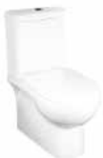
DECINA ADATTO WELS 4 Star 4.5/3L Avg Flush Vol / Soft close, quick release seat / Top and bottom inlet 166645 | BTW Universal Toilet Suite
