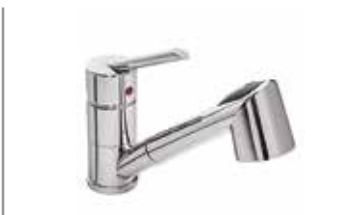
RAYMOR CAPE WELS 4 Star 7.5L/min / Pull-out hand piece / Chrome finish / 191mm swivel spout / 40mm cartridge 133553 | Sink Mixer with Pull-out Spray
